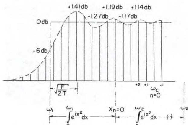
Fig. 8. Method of calculating sideband coefficients for linear sawtooth frequency-modulated carrier with peak angular frequencies  $\omega_1$  and  $\omega_2$ , dispersion  $D = 2\pi F = \omega_2 - \omega_1$ , and sweep time  $T$ .
